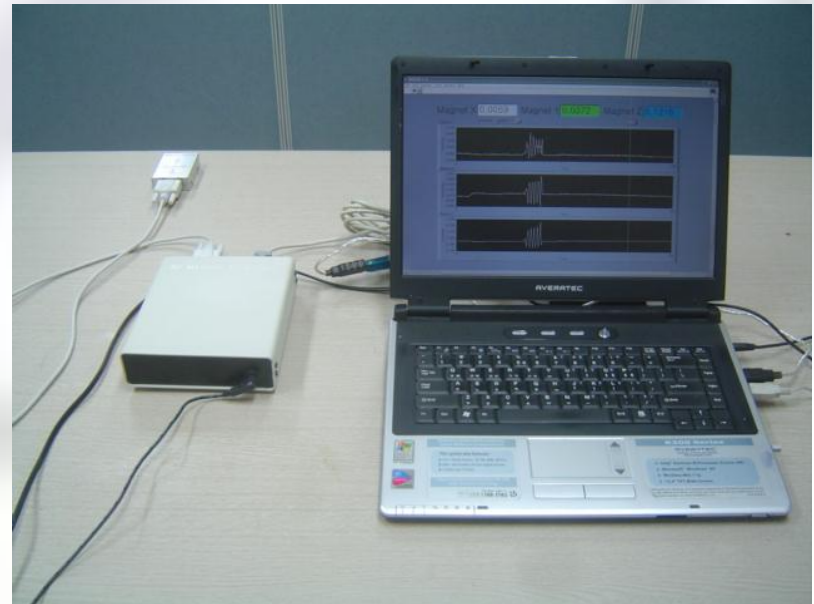
DC magnetic field measurement system
